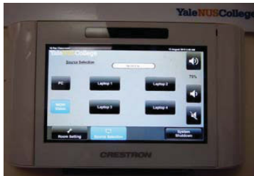
Crestron CP3 remote control and wall mounted touch-panels can be used for accessing various sources such as laptops and PCs in addition to audio levels
